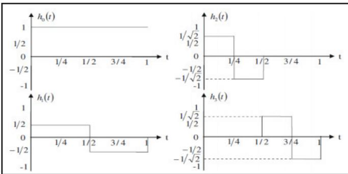
Fig. 1: Haar Wavelets Functions with m = 4.
