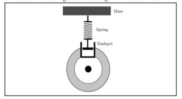
The equation of motion can be described in terms of the vertical displacement x of the mass. Let m be the mass, k dx dt the damping force resulting from the dashpot and nx the restoring force resulting from the spring. Here, k and n are constants. Then the equation of motion is
