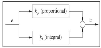
Fig. 3: Block Diagram of PI Controller
