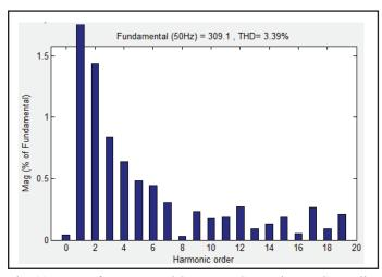
Fig. 11: THD of DVR Based System at Sag Using PI Controller
