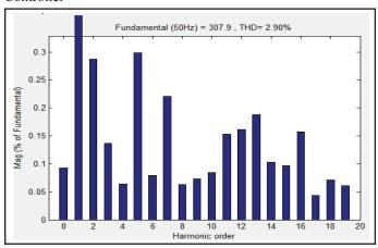
Fig. 14: THD of DVR Based System at Sag Using Fuzzy Logic Controller
