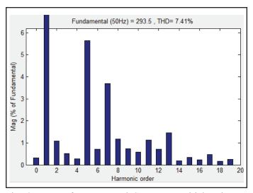
Fig. 9: THD of DVR Based System at Initial Using PI Controller
