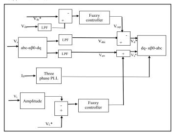
Fig. 6: Self-supported Technique Using SRF Theory
