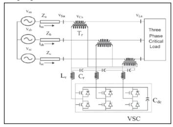
Fig. 1: Schematic Diagram of Proposed DVR System
