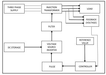
Fig. 2: Block Diagram of Proposed System
