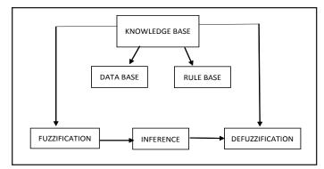
Fig. 4: Block Diagram of Fuzzy Logic Controller
