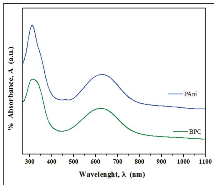
Fig. 3: UV-vis Spectra of PANi and BPC.
