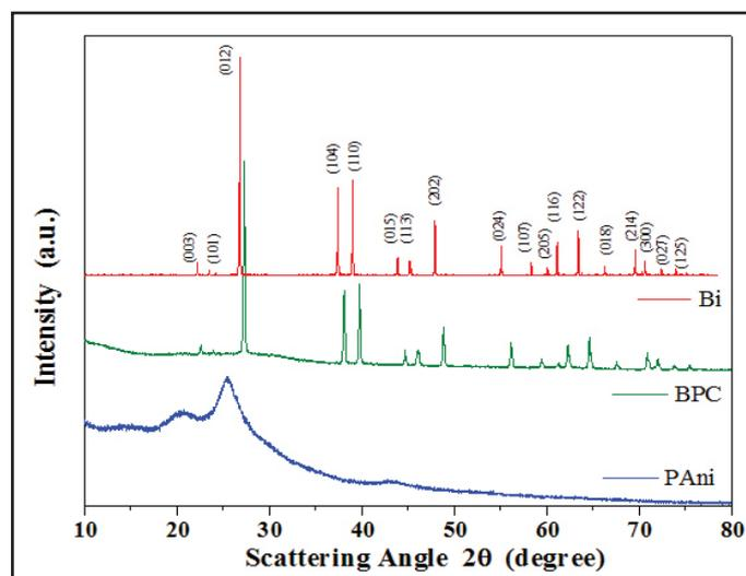
Fig. 1: XRD Patterns of Bi Particles, PANi and BPC.
