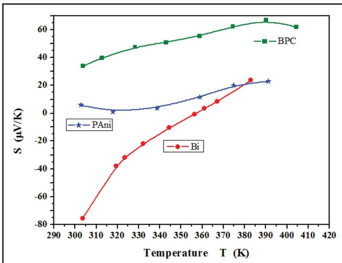
Fig. 5: The Variation of Seebeck Coefficient With Temperature.
