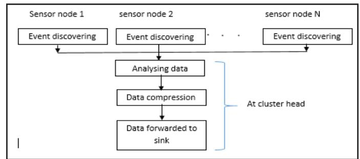
Fig. 3: Process in HCS Super Sensor Method
