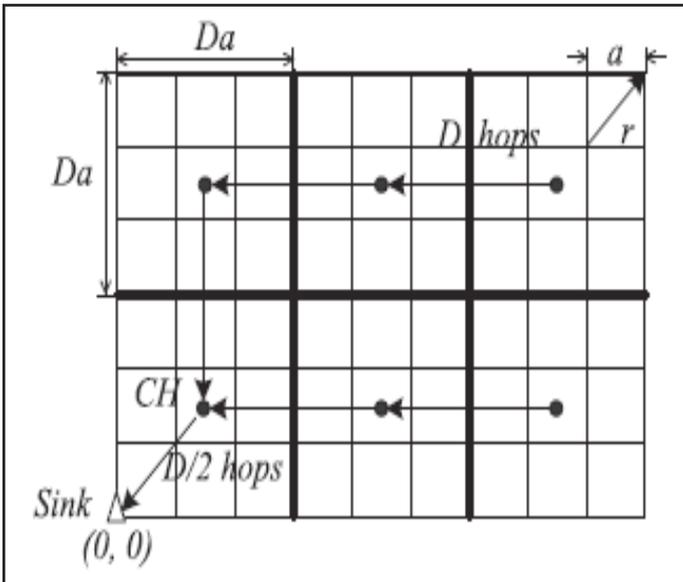
Fig. 4: The Sensor Field is Partitioned Into Small Grids of Size  $a \times a$
