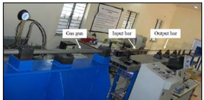
Fig. 5: Split Hopkinson Pressure Bar Used for Present Study
