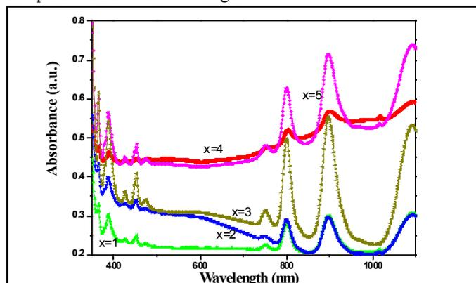
Fig. 2: UV Visible Absorption Spectra of 50P<sub>2</sub>O<sub>5</sub>-10Al<sub>2</sub>O<sub>3</sub>-(20-x) Na<sub>2</sub>O-20CaO-x Dy<sub>2</sub>O<sub>3</sub> Glasses
