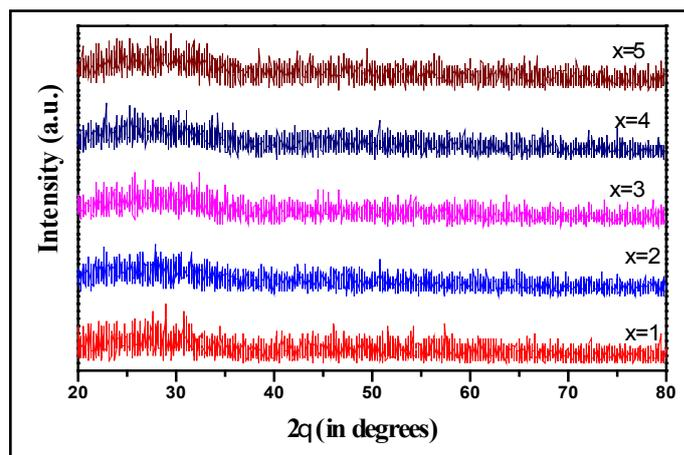
Fig. 1: XRD Spectra of Prepared Glass Samples
