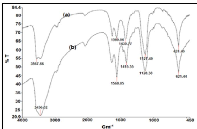
Fig. 6: FTIR Spectrum of La<sub>2</sub>O<sub>3</sub> Nanoparticles Synthesized Using Pechini Method
