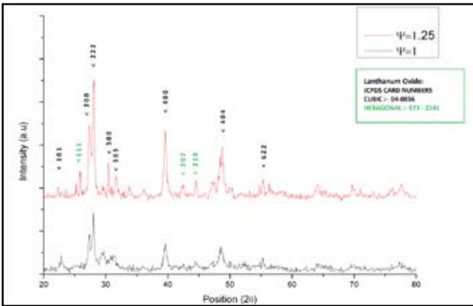
Fig. 1: XRD Patterns of La<sub>2</sub>O<sub>3</sub> Particles Synthesized by Pechini Method for  $\Psi=1$  and  $\Psi=1.25$
