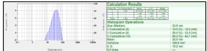
Fig. 3: Particle Size Distribution and Average Particle Size La<sub>2</sub>O<sub>3</sub> Nano Particles Synthesized Using Calculated Using  $\psi=1.25$  in Pechini Method
