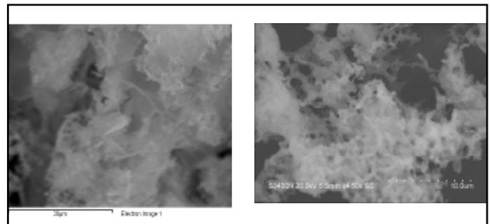
Fig. 4: SEM Images of La<sub>2</sub>O<sub>3</sub> Nanoparticles Synthesized by Maintaining Using Pechini Method Using  $\psi=1$  and  $\psi=1.25$  Respectively
