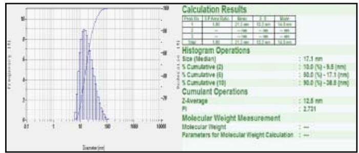
Fig. 2: Particle Size Distribution and Average Particle Size La<sub>2</sub>O<sub>3</sub> Nano Particles Synthesized Using Calculated Using  $\psi=1$  in Pechini Method
