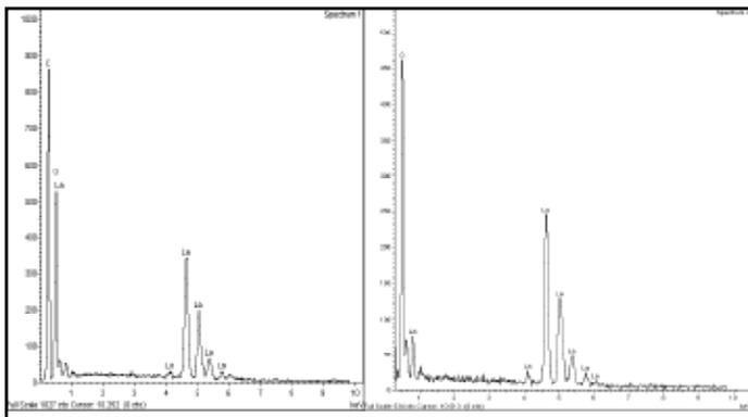
Fig. 5: EDX Pattern of La<sub>2</sub>O<sub>3</sub> Nanoparticles by Pechini Method
