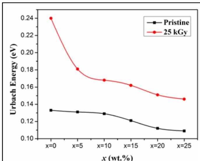
Fig. 5: Variation in Urbach Energy for  $(70B_2O_3-29Bi_2O_3-1Dy_2O_3)-xBT$  Glass Samples With Absorbed Dose and Weight Fraction of BT
