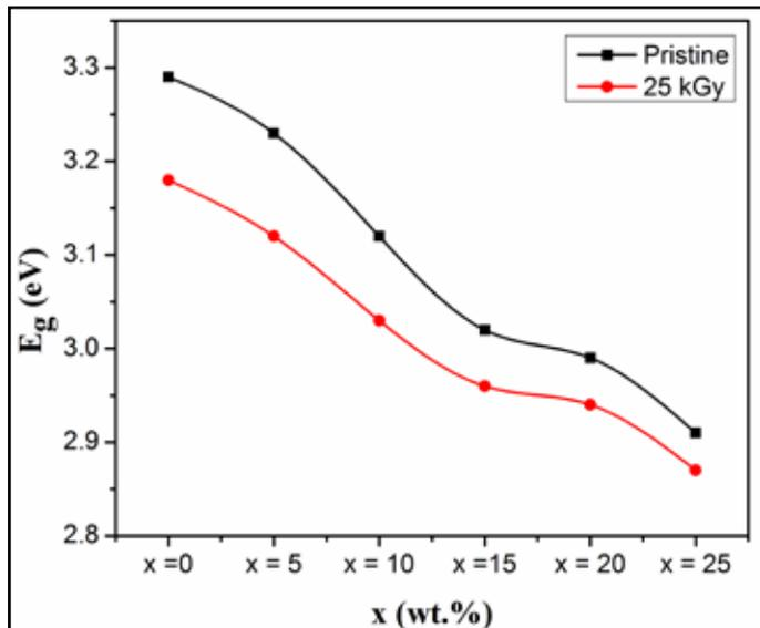
Fig. 4: Variation in Band Gap Energy for  $(70B_2O_3-29Bi_2O_3-1Dy_2O_3)-xBT$  Glass Samples With Absorbed Dose and Weight Fraction of BT
