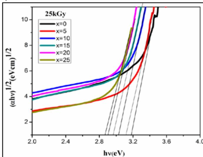
Fig. 3: Tauc's Plot for  $(70B_2O_3-29Bi_2O_3-1Dy_2O_3)-xBT$  Glass Samples After Irradiation
