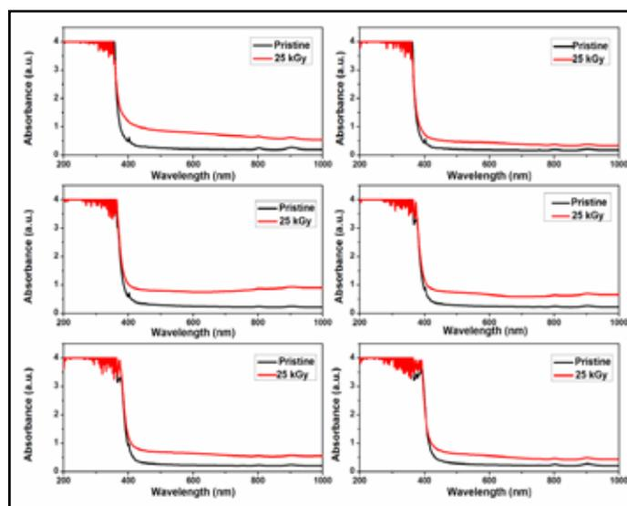
Fig. 1: Optical Absorption Spectra of BT-doped Bismuth Borate Glasses With Increasing BT Content Before and After Gamma Irradiation
