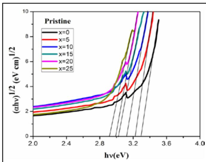
Fig. 2: Tauc's Plot for  $(70B_2O_3-29Bi_2O_3-1Dy_2O_3)-xBT$  Glass Samples Before Irradiation.
